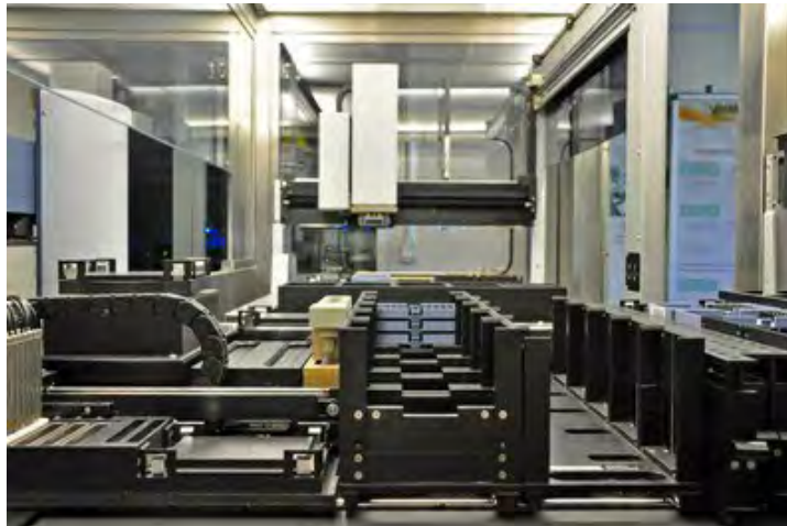
Robotic platform with high-throughput liquid handler for sample dilution and treatment.
